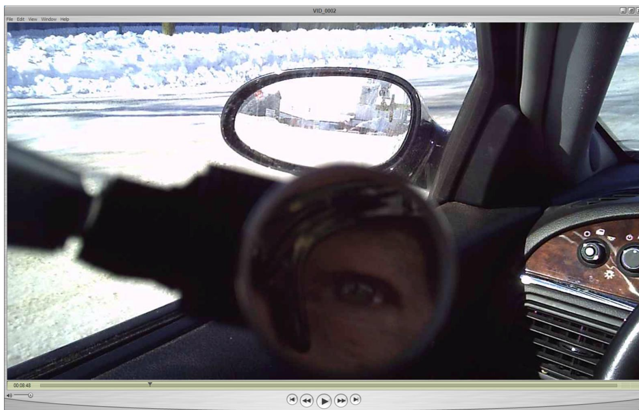
Figure 25: View from video eyeglasses when the test driver looked toward the driver's exterior mirror. The view of the pupil of the driver's right eye is visible in the small mirror in the bottom centre of this figure.
