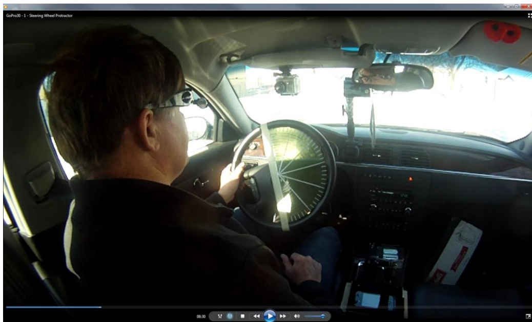
Figure 21: View from GoPro30 showing the protractor attached to the steering wheel hub to document the speed and magnitude of steering wheel rotation.
