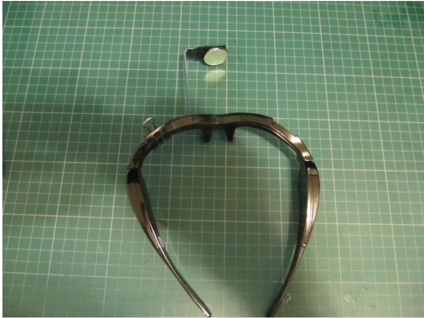
Figure 17: View of video eyeglasses with an attached mirror used to document the motion of a driver's right eye.
