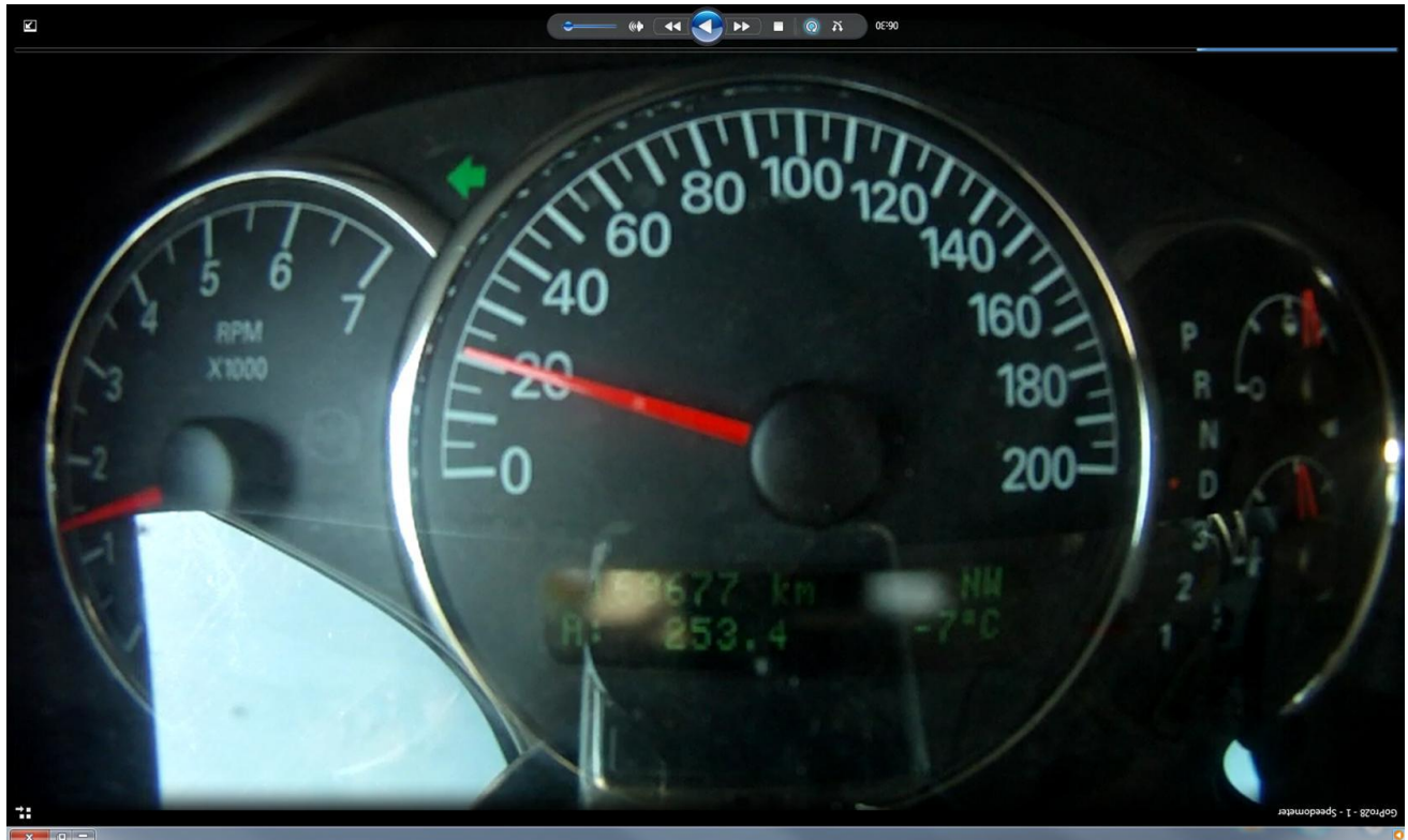
Figure 22: View from GoPro28 showing the instrument cluster of the test vehicle. In the present view the test vehicle is travelling about 21 km/h, the tachometer reads about 1300 rpm and the left turn signal is activated. The outside air temperature reads -7 C.
