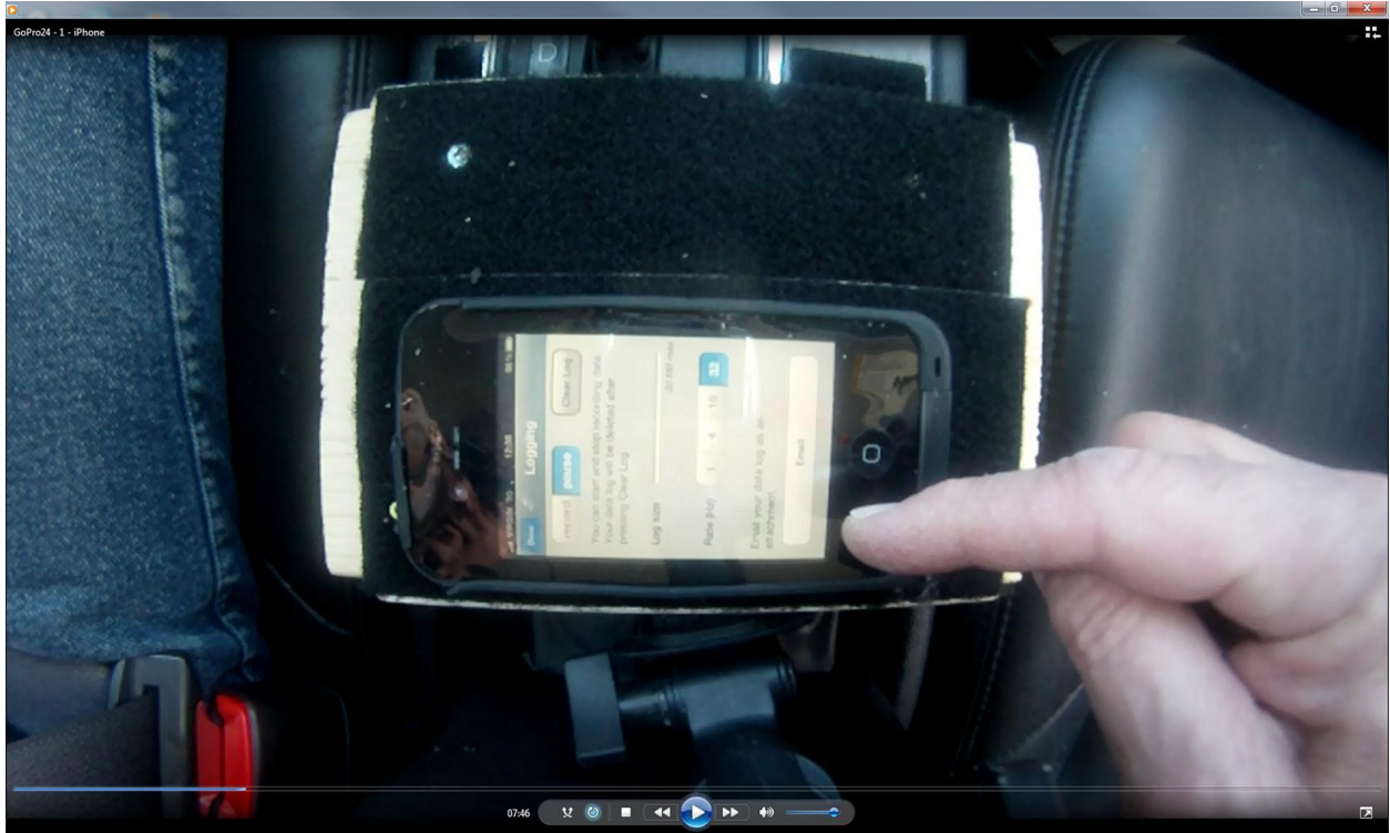
Figure 24: View from GoPro24 showing the face of the iPhone as it is being set-up to start recording of the readings from its accelerometer.
